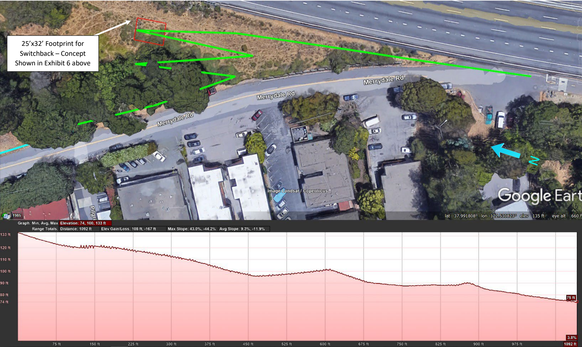
Exhibit 9 - Plan and Profile - Grade to slope no greater than 5%
