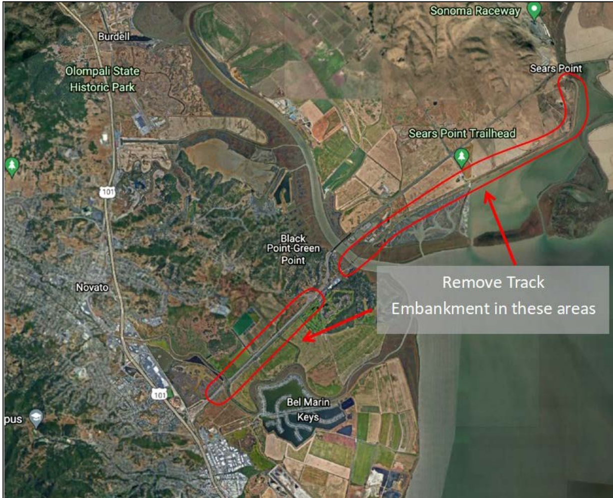
Figure 17. Track and Embankment Removal Area to Allow Bay Restoration
