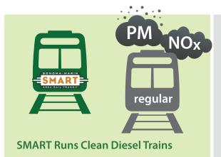
SMART's clean-diesel trains have modern, efficient engines that meet the EPA's Tier 4 emission standards, cutting particulate matter emissions by 96% and NOx emissions by 93% compared to regular diesel engines.
