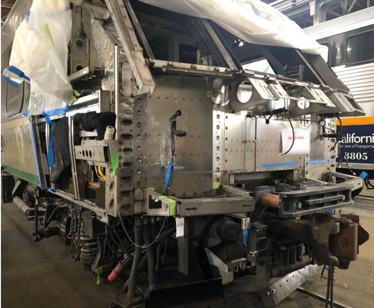
The SMART fleet is undergoing modifications to the drivetrain in order to prevent issues discovered on Metrolinx fleet in Toronto.
